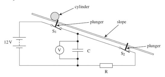
$S_1$  and  $S_2$  are two switches that would be opened in turn by plungers as the cylinder passed over them. Once opened, the switches would remain open. The cylinder would be released from rest as it opened  $S_1$ . The pd across the capacitator would be measured by the voltmeter.
